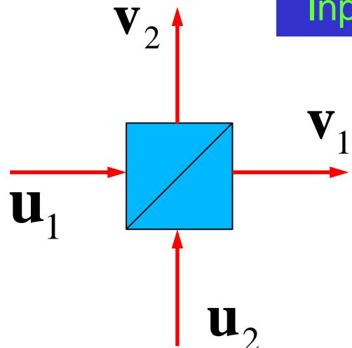
Input-output modes of a beam splitter
