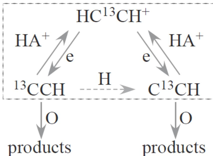
$$\frac{[\text{C}^{13}\text{CH}]}{[^{13}\text{CCH}]} = \frac{2k_{ex}^{(f)}[\text{H}] + k_d[\text{O}]}{2k_{ex}^{(b)}[\text{H}] + k_d[\text{O}]}$$
