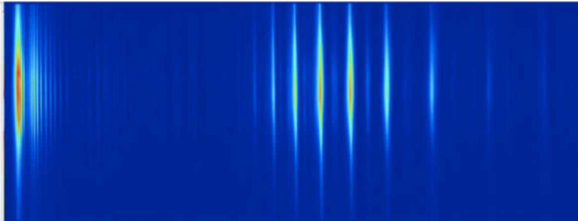
HHG spectrum in argon with a transmission spectrometer
