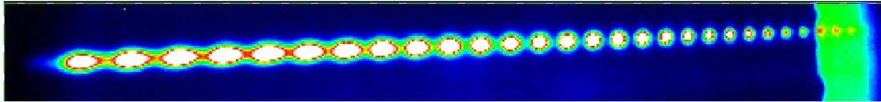
HHG spectrum in neon with an imaging spectrometer
