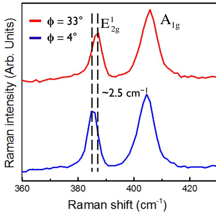
Biaxial uniform tensile strain
