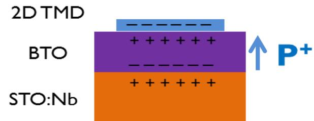
WS<sub>2</sub>/BaTiO<sub>3</sub>: before annealing
